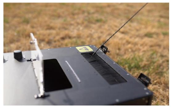
9. When the cable reaches the limit length, the alarm will be triggered (press the power switch, the alarm will be cancelled). Do not fly higher. Lower the drone.
