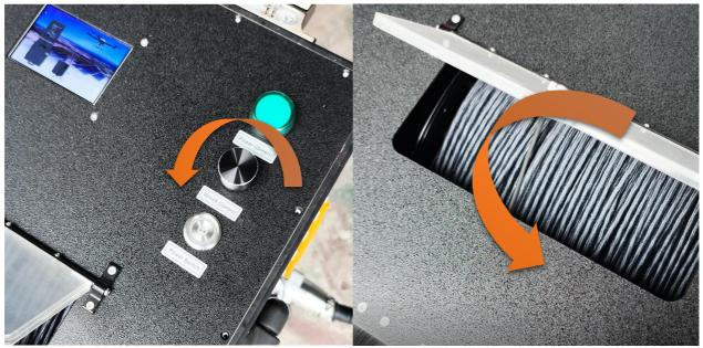
Attention. Watch the tension of the tether. Keep the tether not too tight in case of drop-down of the drone.
